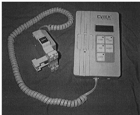
The electro-digital inclinometer EDI-320.
