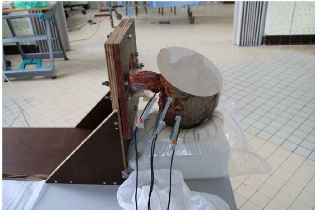
FIGURE 1. Experimental set-up: specimen in supine position with the Zebris system.
